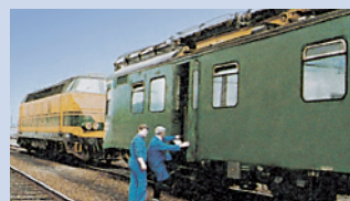
Overhead line inspection railcar
